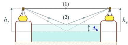
Fig. 1: The two-ray model showing: (1) the direct LoS ray, and (2) the indirect ray reflected from the surface when experiencing a water level variation of  $\Delta_k$ .
